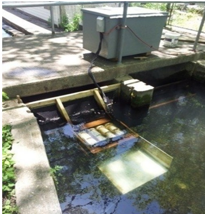
Figure 2.3. Smith-Root 1601 counter with 8 four-inch diameter tunnel counting array installed with 110 V power at the Benoit's Pond fish ladder exit on the Monument River, Bourne.
