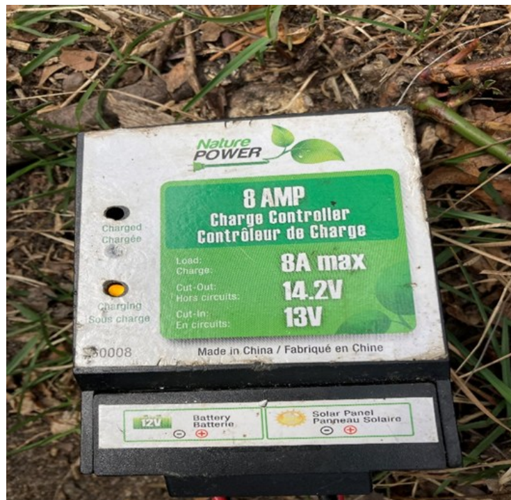
Figure 2.6. Example of suitable solar charge controller for electronic counters.
