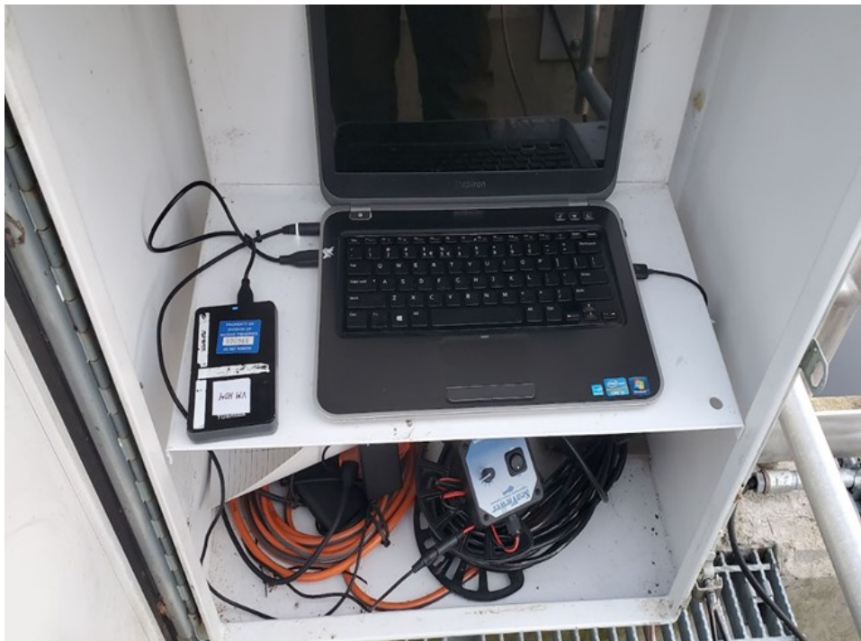
Figure 3.5. McCallister enclosure box with laptop, external hard drive, and SeaViewer 950 video camera cable.
