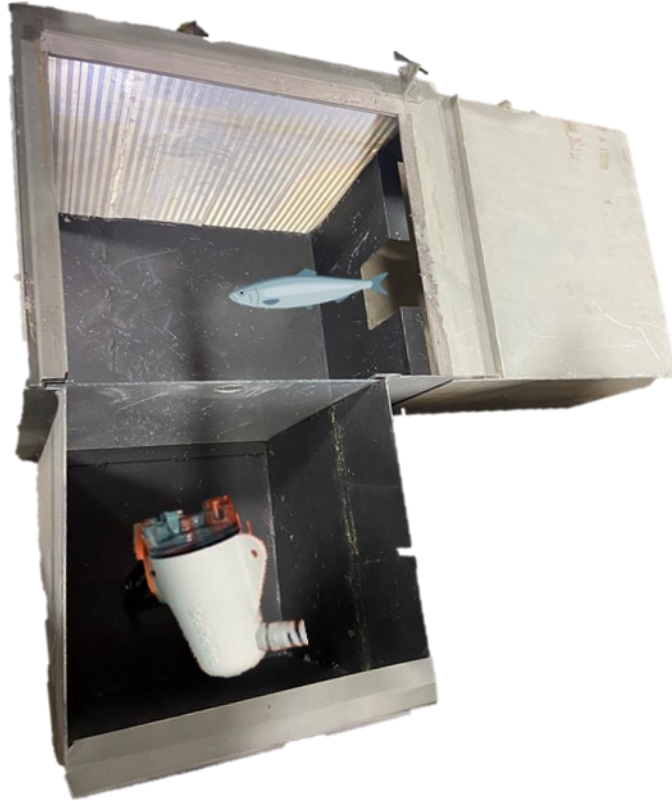
Figure 3.3. Custom fabricated aluminum video camera housing attached to fishway exit board slots.
