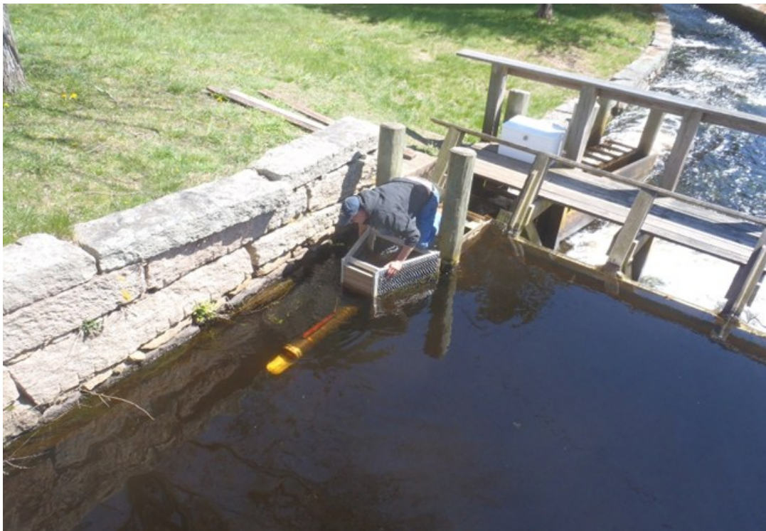
Figure 2.1. Single tube counter installed at exit of Alaskan Steeppass fishway at Sippican River, Rochester, MA.
