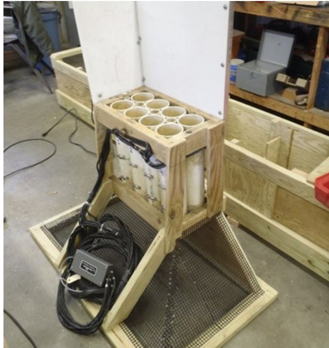
Figure 2.2. Eight-tube counter for Monument River, Bourne, MA. Early test model with wood frame. An improved design was later deployed with a fabricated aluminum frame.
