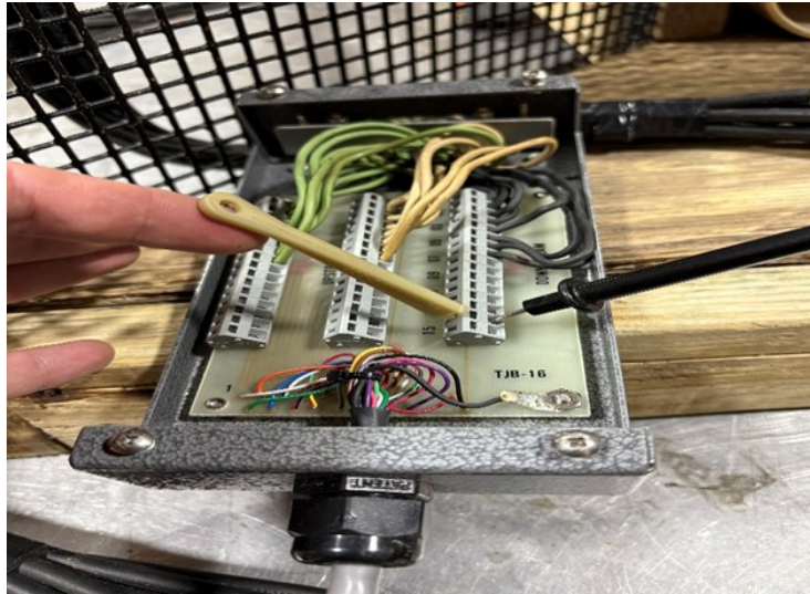
Figure C.4. The custom tool is being used to open a terminal to insert the prong to test resistance with the multimeter.
