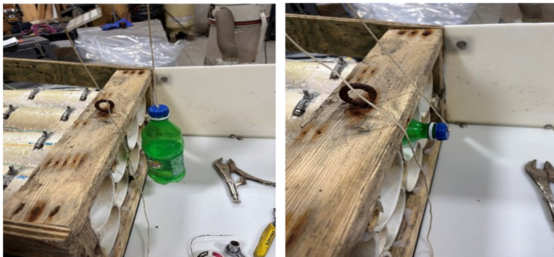
Figure C.1. A soda bottle being used to test whether a tube is working properly. The bottle is attached to a string, then pushed through the tube while holding on to the string.
