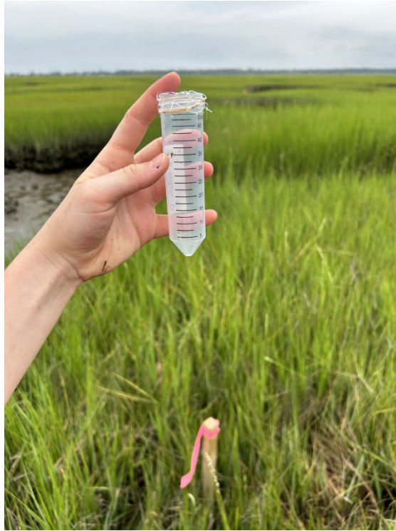
Figure 3: Example of a sediment trap pre-deployment at Chase Garden Creek.
