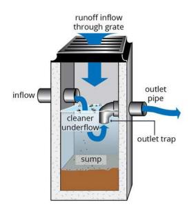
Unmanaged stormwater contributes to poor water quality in our ponds by conveying nutrients and contaminants. While the traditional catch basins do little or nothing to treat stormwater, they do help control the flow and help to capture and settle out sediment and litter—that is if they are maintained and properly functioning.
