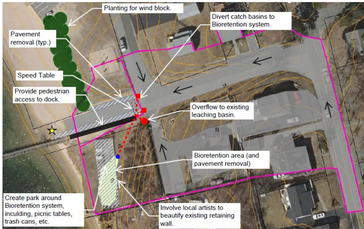
Site Sketch: Drainage area (pink), impervious cover (gray), impervious cover reduction (striped gray), BMPs (light green), paved flumes (dark blue), proposed infrastructure (red), revegetation (dark green), and drainage flow paths (arrows). Star represents the GIS location of the boat ramp.
